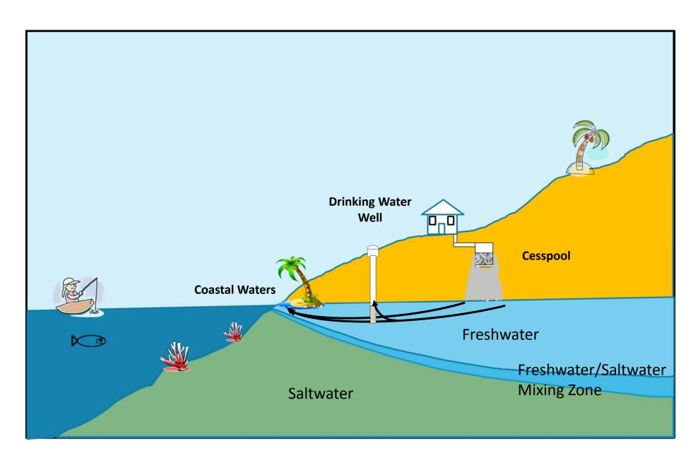
Cesspool leachate seeps into the groundwater then is transported down gradient to wells and to the shoreline
